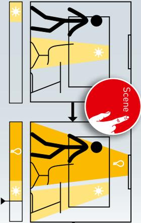
If the default scene contains presence detection with semi-automatic operation, the scene is started with a push-button or with a tablet or smart phone.
