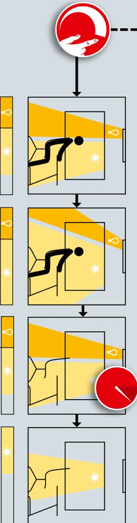
In the case of a manual intervention, the dimming and switching of luminaire groups, the constant light control is deactivated for these luminaire groups. During the stay in the room, the changed dimming levels of the lighting scene are retained.
