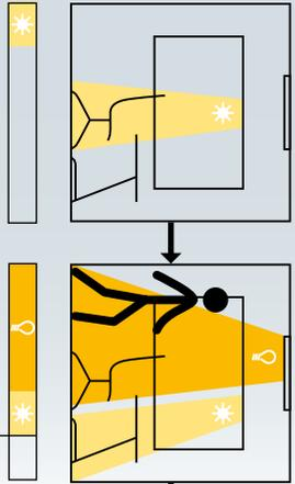
If the default scene contains presence detection with fully automatic operation, the lighting starts with the default scene upon entering the room.
